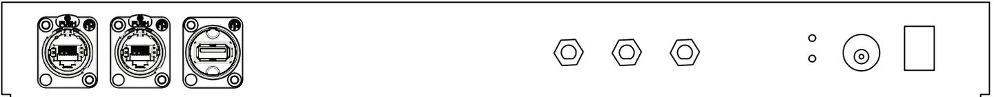
Back panel includes: (2) Ethernet; USB; Wifi; GSM; GPS antenna connection;
