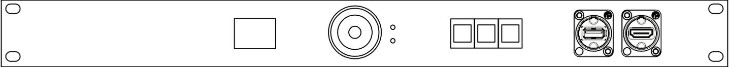
Front panel includes: Small OLED Display; Selector wheel; (3) User-programmable buttons; USB; HDMI
