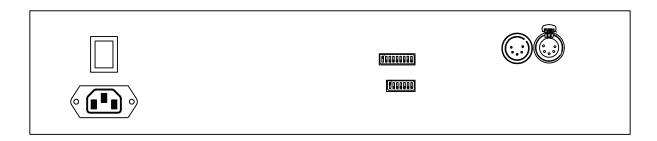
Back panel includes: Main power switch; IEC power connector; Dip switches to set start address and mode; XLR 5-pin thru and out DMX
