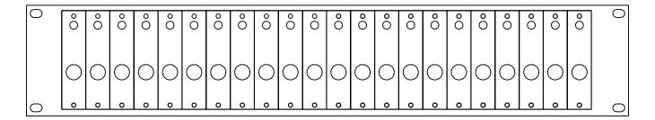
Front panel includes: Space for 22 switch plates (maximum 24 switches)
